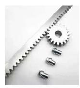
The sliding gate gear rack is made of Q235 material. The module 4 gear rack are popularly used on the sliding gate, driven by the reducer and gear, the gear rack soldered on the gate can be pulled and pushed to slide on the track. The zinc plated finish can make it rusty proof.
