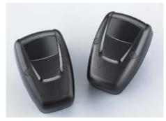
This photocell is designed to detect obstacles in automatic door and gate installations, preventing collision with the door/gate. They are made up of an infrared transmitter module (TX) and receiver module (RX). If a person or object interrupts the beam of light emitted by transmitter (TX) (or the beam does not reach the receiver due to failure or loss of setting), the receiver (RX) enables the corresponding relay sending signal to control unit to keep the door & gate open.
